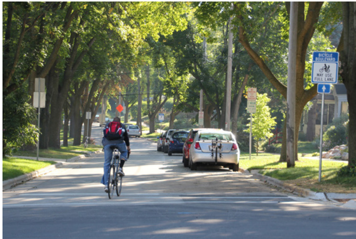
Figure 1. Photo Source: NACTO A street segment, or series of contiguous street segments, that has been modified to accommodate through bicycle traffic and minimize through motor traffic.
