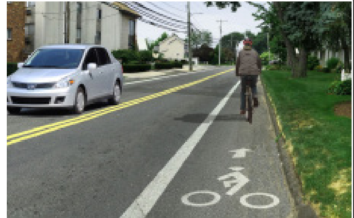
Figure 3. Photo Source: FHWA A portion of roadway that has been designated for preferential or exclusive use by bicyclists by pavement markings and, if used, signs. It is intended for one-way travel, usually in the same direction as the adjacent traffic lane, unless designed as a contra flow lane.
